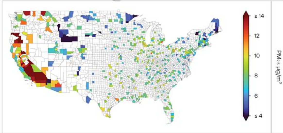
Figure 1a: A map of the contiguous United States with county-level annual design values from 2020-2022 and sourced from the 2022 EPA design value report for fine particulate matter.
