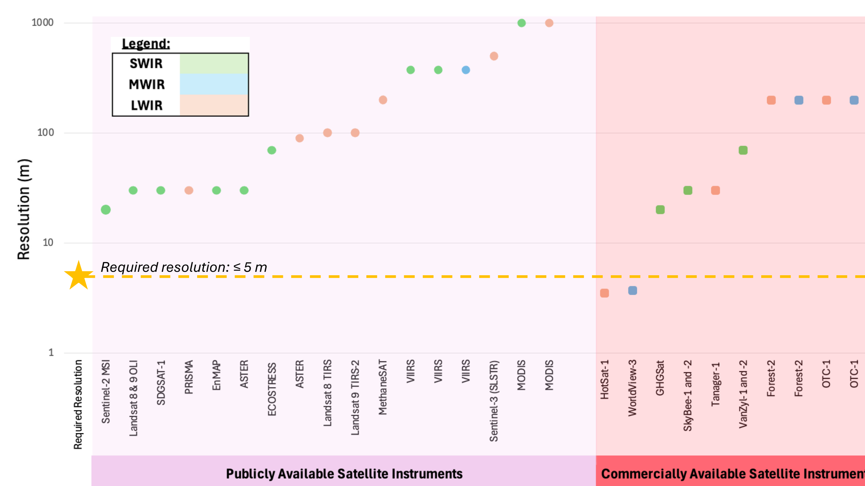
Figure 3: An inventory of the various publicly (purple) and commercially (red) available satellite instruments, plotted based on their individual spatial resolutions (m). The instruments are color-coded based on their wavelengths: short- (SWIR, 1.4-2.5 \mu\text{m} , green), medium- (MWIR, 2.5-7 \mu\text{m} , blue), and long-wave (LWIR, 7-15 \mu\text{m} , orange) IR (Desta et al., 2020). The ideal resolution of \leq 5 m is plotted as a yellow star on the far left. Each instruments' operational information was obtained from the ESA's eoPortal site.
