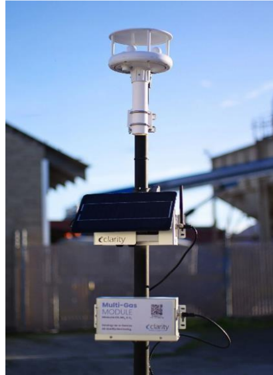
Clarity Node sensor measures Particulate Matter, Nitrogen Dioxide, Ozone, and meteorological data
