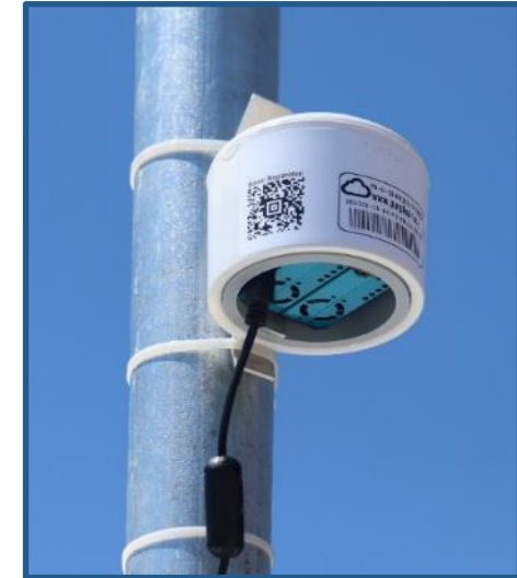
Purple Air Sensor measures Particulate matter, temperature, and humidity
